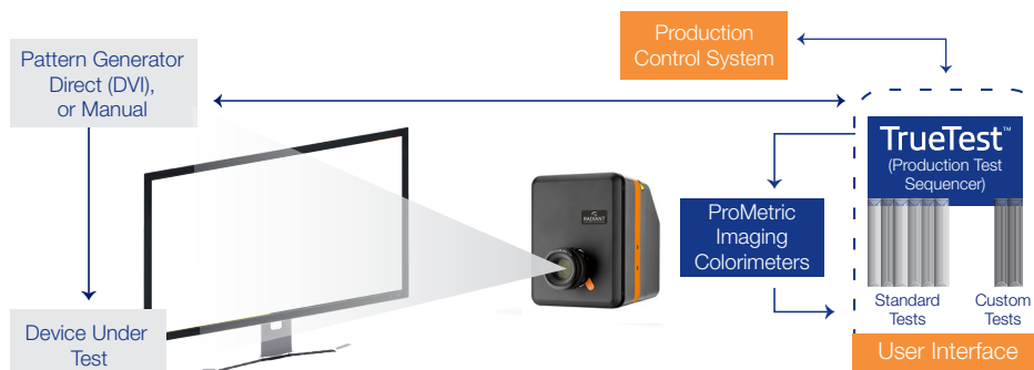
Figure 1 - FPD AVI test set up with an imaging colorimeter under automated software control.
