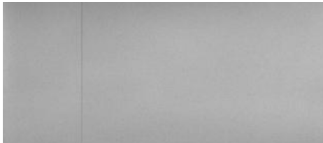
Figure 2 - Photopic measurement of a display screen with a line defect visible.
