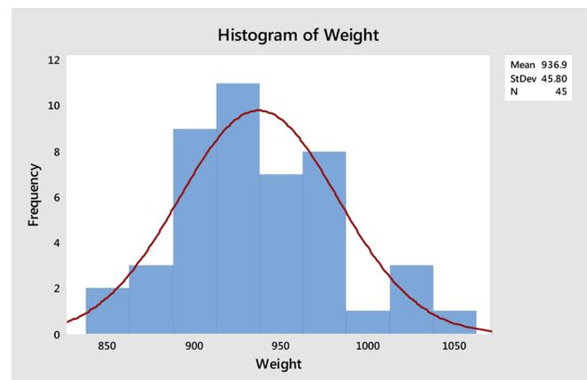
A histogram provides a snapshot of numeric, continuous data. With histograms, you can quickly identify the center and spread of your data. Where does most of the data fall? And where are the minimum and maximum values, approximately? A histogram also shows you if your data are bell-shaped or not, and can help you identify outliers, or highly unusual data points, which may require further investigation.
