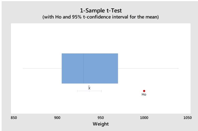
A t-test can be used to compare the average of one sample to a target, or to the average of another sample. For example, if your company sells beverages in 16 oz. containers, you can use a 1-sample t-test to determine if your production line's average fill is off target. If you buy flavor syrup from two suppliers and want to determine if there's a difference in the average volume of their respective shipments, then you can use a 2-sample t-test to compare the two suppliers.
