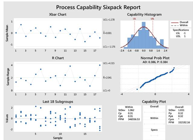
Nearly every process has an acceptable lower and/or upper bound. Manufactured parts can't be too large or too small, wait times can't extend beyond an acceptable threshold, fill weights need to exceed a specified minimum. Capability analysis quantifies how well your process meets specifications, and provides insight into how to improve a poor process. Frequently cited capability metrics include Cpk, Ppk, defects per million opportunities (DPMO), and Sigma level.
