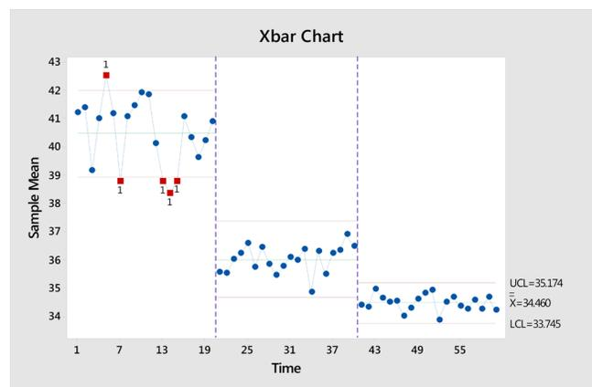
A stable, and therefore predictable, process is a hallmark of quality products and services. Yet every process has natural fluctuation. A control chart distinguishes "special-cause" variation from acceptable, natural variation. These charts graph data over time and flag out-of-control data points so you can detect unusual variability and take action only when necessary. Control charts also help you ensure that your process improvements are sustained into the future.
