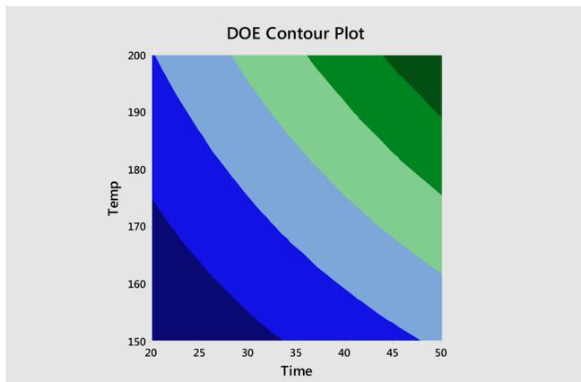
While regression and ANOVA are typically used for data that's already available, Design of Experiments (DOE) provides an efficient data collection strategy, where inputs are simultaneously adjusted, to identify if relationships exist between inputs and outputs. Once you collect the data and identify the important inputs, you can then use DOE to determine optimal settings.
