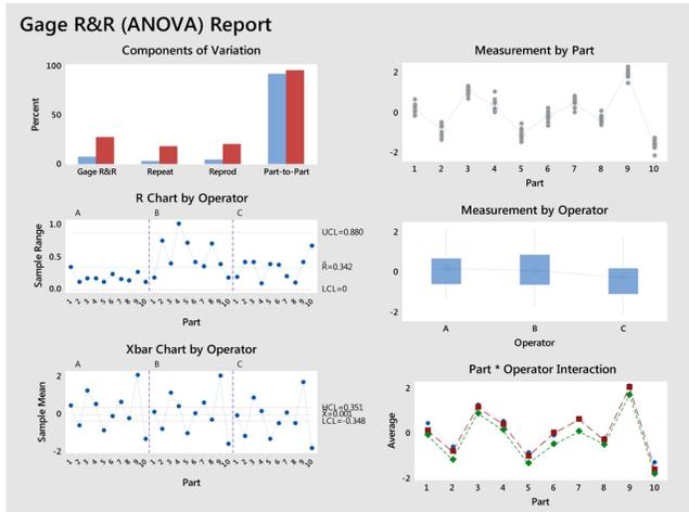
Would you weigh yourself using an unreliable scale? Would you wear a watch that didn't keep time? You can't improve a process that you can't adequately measure, which is why we need Gage R&R. This tool—for continuous numeric measurements, such as weight, diameter, and pressure—helps you determine if your measurements are both repeatable and reproducible, when the same person is repeatedly measuring the same part, and when different operators are measuring the same part.
