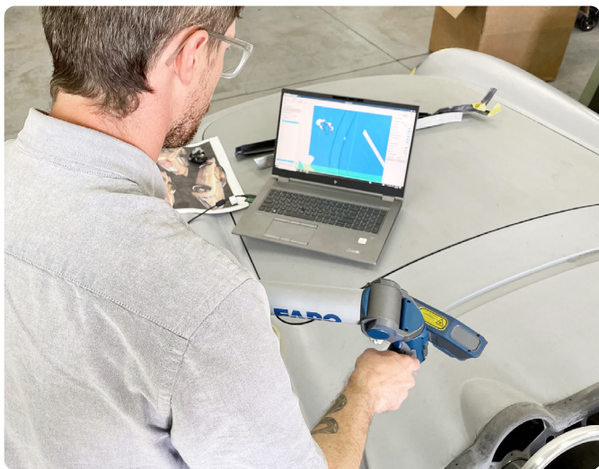
Greg Hebard scanning a 1953 Kindig CF1 for reverse engineering purposes
