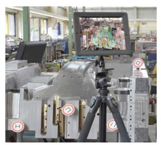
With the tablet's integrated camera, an overlay of the as-built object with virtual 3D data, including all process and workflow information, can be realized in real time.
