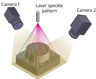
figure 3: Active stereo example using laser speckle pattern to create texture on object.
