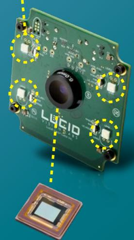
Sony DepthSense IMX556PLR CMOS with 6mm lens
