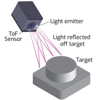
figure 7: ToF systems have a light source and a sensor.
