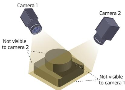
figure 2: Occlusion occurs when a part of an object cannot be imaged by one of the cameras.
