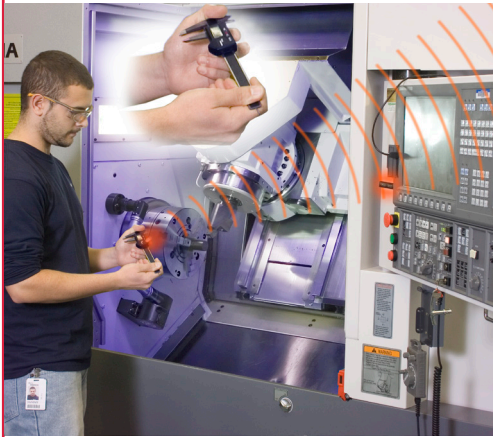
Integrated wireless is ideal for point of manufacture inspection, making measurements directly in the machine with immediate feedback to the machine controller.
