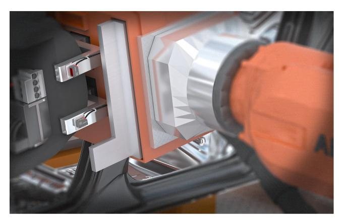
Car body positioning in the production line: For automated processing of car bodies or vehicles, e.g. for drilling, punching and subassemblies, an exact determination of the position relative to the processing tool is necessary.
