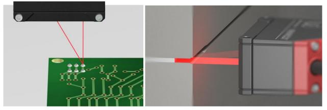
Small light spot for demanding applications: The extremely small light spot monitors even finest pin geometries reliably while measurements can be carried out in limited spaces.
