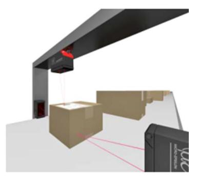
Dimensional inspection: In fully-automated logistics processes, the dimensions of packages are checked. Due to their large measuring range and their high measuring rate, compact laser sensors from Micro-Epsilon are used for automated, dimensional inspection.
