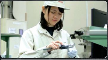
Final inspection data not only certifies the part for conformance but also predicts the conformance of future parts manufactured. This data can be collected and compared to data measured at the point of manufacture or data collected during audits.
