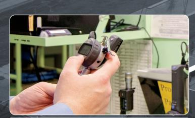
Inspection being performed at the point of manufacture. Sampling techniques based on capability reduce the time spent on inspection while still ensuring the quality of the product.
