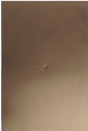
Fig. 3 Specimen After Impact Test (30.5 J Impact Energy)
