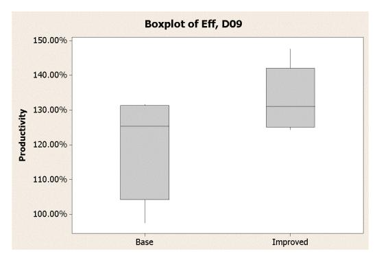
The boxplot above shows the overall productivity level both before and after the improvement solutions were implemented for the departments responsible for producing the 2.5-inch steel tubing.
