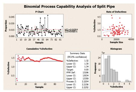
The project team at Tenneco performed process capability analysis in Minitab at the onset of their project to assess process variation.
