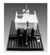
by self-wedging tension clamps or some other similar method. These items can be fastened in an almost unlimited number of different ways in order to hold thousands of different parts. A set of modular tooling large enough to hold tabletop sized parts usually requires a relatively small upfront investment usually on the order of \$5,000 or less.
