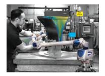
Points in space are digitized by touching the probe to a feature and pushing a button to capture the point's location. The sphere's diameter is known with a high degree of certainty which allows the software to account and compensate for it. This ensures that features such as diameters of holes are measured accurately and do not add the probe diameter to the measured value.
