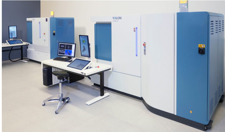
YXLON FF20 CT and FF35 CT Nondestructive Test Inspection Systems
