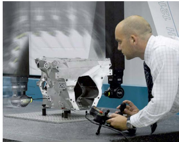
5-axis scanning allows fast, seamless inspection of complex components, without pauses for indexing and stylus changing.
