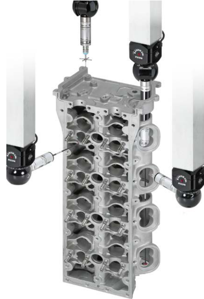
Flexible, modular sensors and indexing heads can increase measurement flexibility and automation, providing access to all component features in a single set-up.
