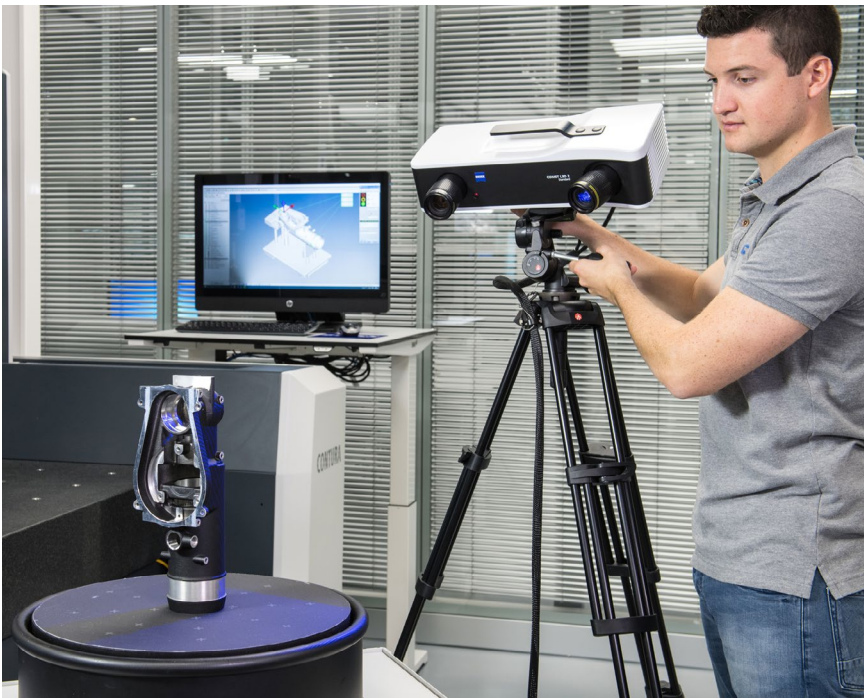
COMET captures millions of measurement data points in as little as one second with fringe projection technology.
