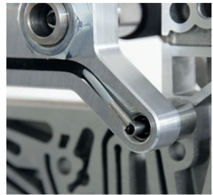
Companies can save a half hour per eight-hour shift if the workpiece temperature is captured automatically with an integrated temperature sensor in the pallet.
