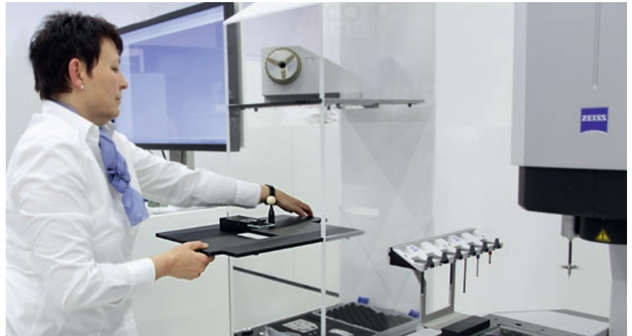
Pallets reduce downtime: while the measuring machine is still measuring, operators can stage the next set of workpieces to be measured onto the pallet. Calibration pallets with a fixed reference sphere mount and sphere save additional time.
