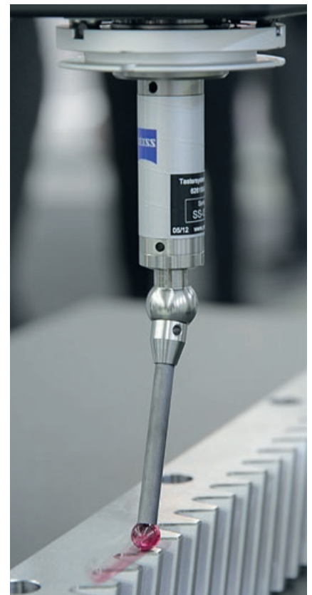
Special software options like ZEISS 'FlyScan' can cut the measuring time in half. These enable e.g. the stylus to travel over spaces in the surface more quickly during the scan.
