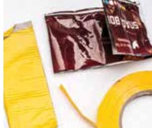
Adhesive strength properties are measured to understand the bonding capabilities of coatings and glues on various types of materials- from paper to substrates to building materials. Both 90° and 180° testing can be performed to measure the peak holding strengths under standard test methods such as ASTM F88.
